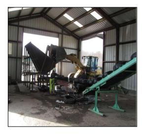
The shredding of tires started in 1988. Employees derim tires on site and recycle the rims. Tires are then processed through the tire shredder. The finished product is used as supplemental daily landfill cover, and used in drainage projects, pipe substrate, road base material and to repair seeps in landfill slopes.
